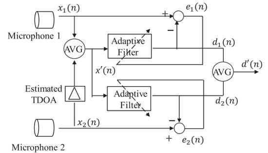
Fig. 4. Basic scheme of adaptive signal enhancement filter in proposed system.
