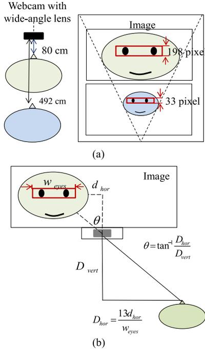
Fig. 5. Illustration for estimating (a) distance and (b) angle of desired speaker.
