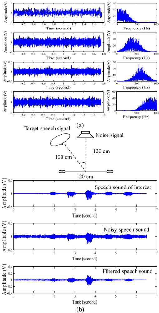
Fig. 10. (a) Four types of Gaussian noises and their power spectrums. (b) Speech sounds of interest, noisy speech sounds, and filtered speech sounds under non-stationary noise.
