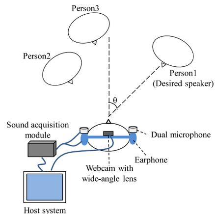
Fig. 1. Basic scheme of proposed hearing aids with image recognition technology.
