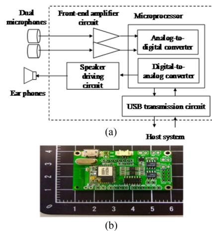
Fig. 2. (a) Block diagram and (b) photograph of sound acquisition module.
